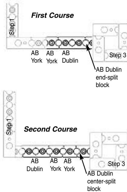
Figure 4: 1st Wall Panel Layout
