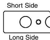
Place a Corner block along the guideline at the corner location with the long side facing out (Figure 2). Then, split an AB Dublin end-split block along the splitting notch and place the large piece with the split side against the Corner block (Figure 1). Splitting the block creates a straight edge so there will not be a gap where the blocks meet. See *How-to sheet #210* for more information on splitting blocks.
