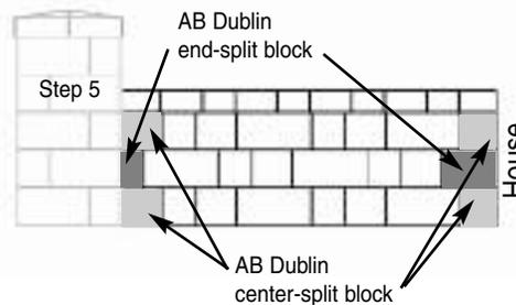
On the second course, split an AB Dublin end-split block and place the large piece with its split side against the house. Save the small piece to use at the end of this course. Continue stacking the wall panel to the next post/pillar location using the pattern you have chosen, ending each course with the remaining split block used at the beginning of that course, with split side facing out
