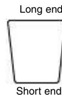
Next place Wall Cap (B) on the other side of the corner. Place the short end of the Wall Cap facing the outside of the wall. Make adjustments as necessary to ensure they line up properly at the corner.
