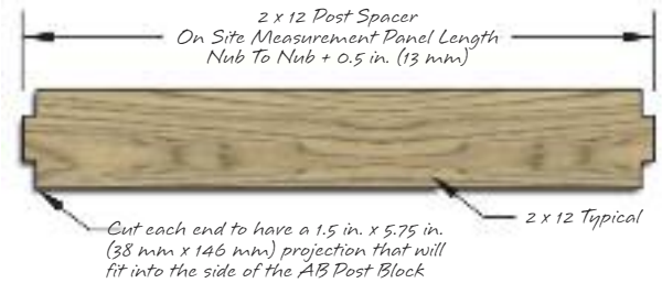
Figure 4: Post Spacer Jig
