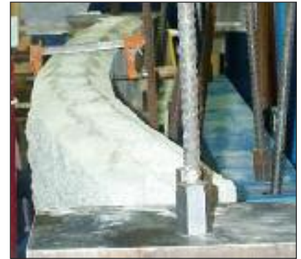
Top bond beam deflection.
