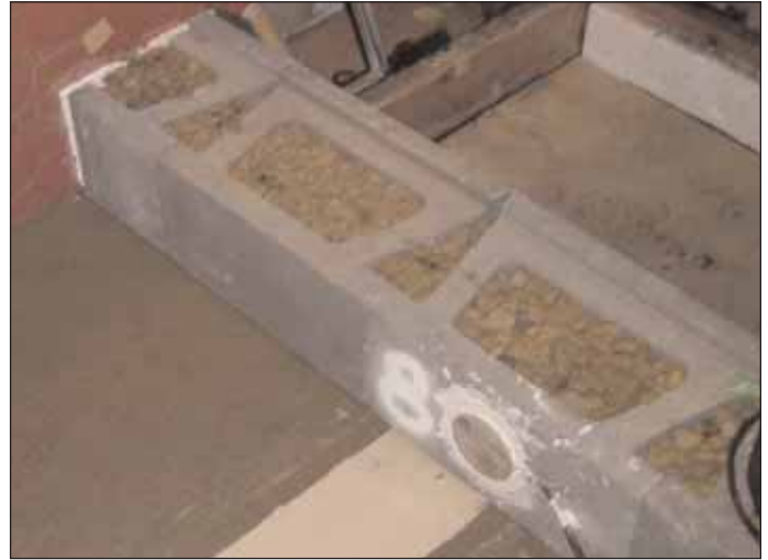
A Layer of White Sand Seam Used to Identify Post-Test Shear Location
