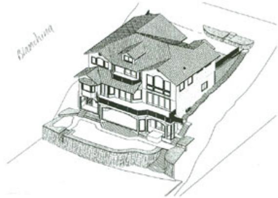
The prominent design challenge on these projects is that most of the walls are located near the shoreline. City requirements do not allow any walls to be built below the high water elevation of 510.0 feet (155 m). Therefore it was critical that each of the walls be laid out with careful consideration to the bottom of wall elevations and grading in order to receive a building permit.
