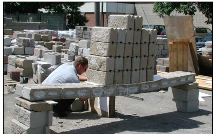
Figure 2: Loaded 7 Panel Bond Beam
