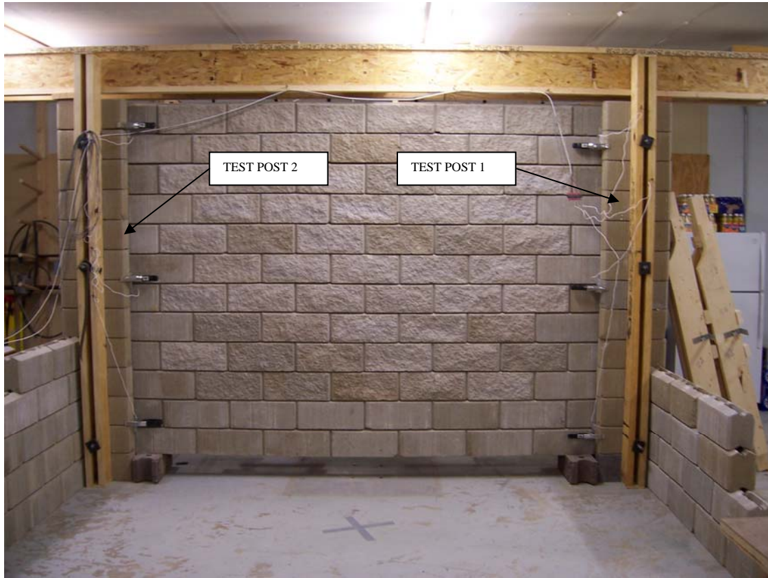
Figure A6: Full-Scale Panel Set-up showing Post 1 and 2
