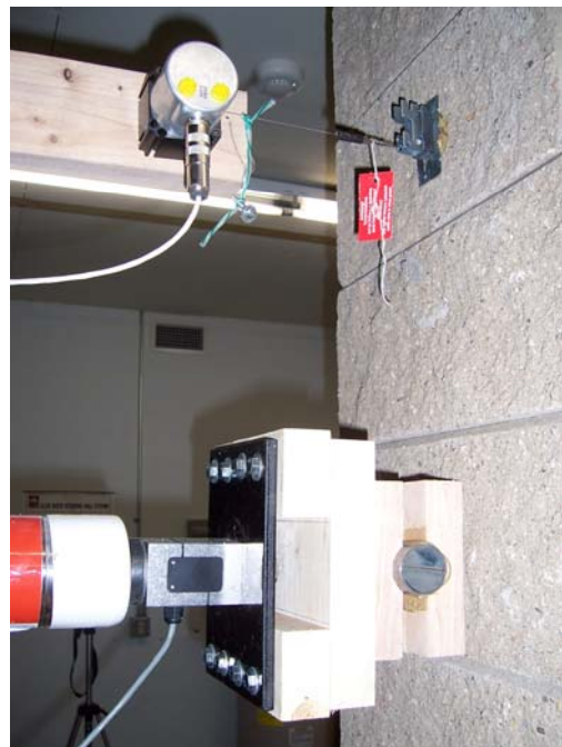
Figure 2: In Place Load Cell and Deflection Transducer
