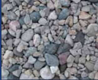
Wall Rock makes compaction easy around the blocks and locks them tight together. It also acts like a filter, keeping the fine-grained soil from bleeding through the face of the wall.
