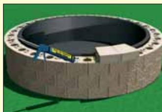
Place the liner inside the ring of blocks. Position the Wall Caps and glue them down with concrete adhesive. This will lock the blocks together and prevent unwanted disassembly.
